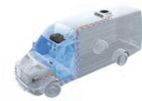
Evaporator integrated into the roof
