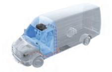
Evaporator integrated into the roof
