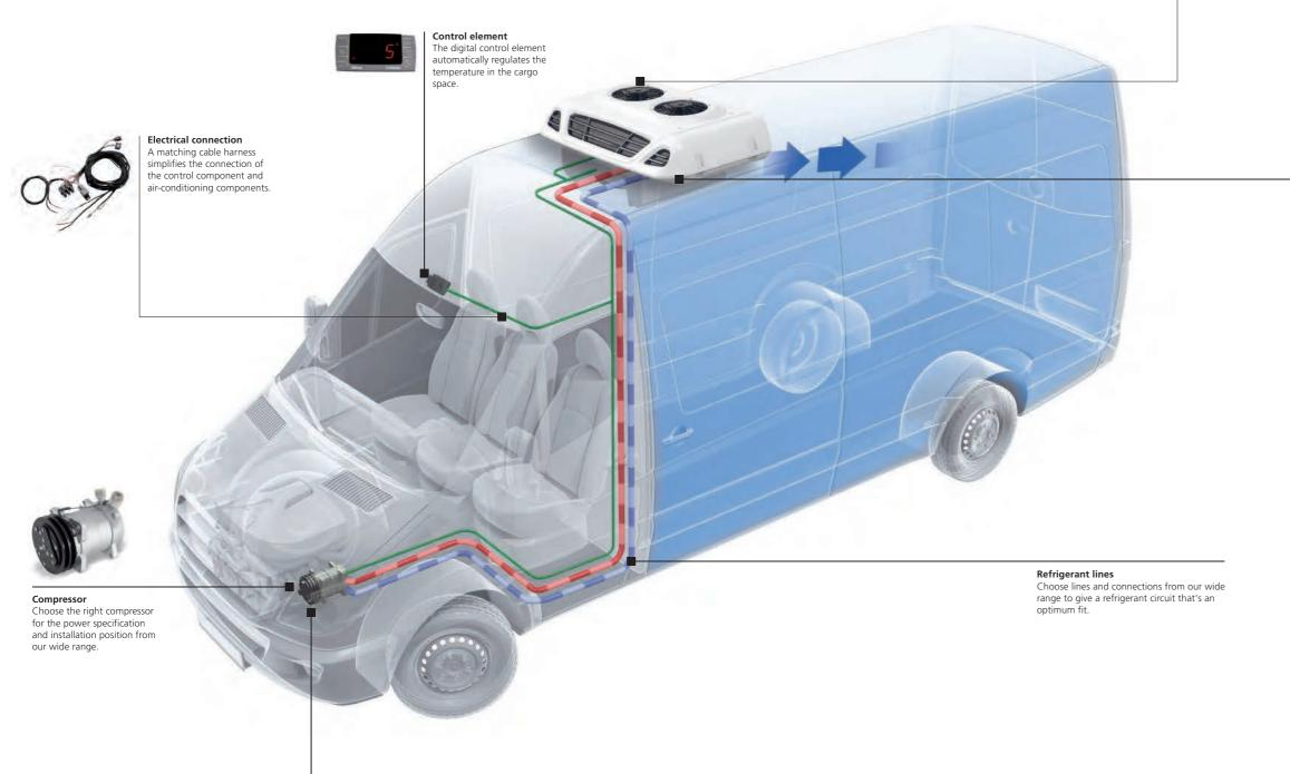
**Installation kit for compressor** Vehicle-specific installation kits ensure easy fitting and reliable operation of the compressor. This function ensures continuous operation, even when stationary.
