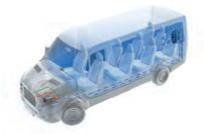
Evaporator under the roof
