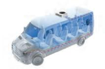
Evaporator under the roof
